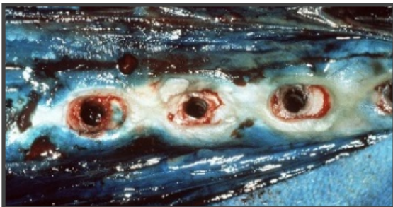
Fig. 3: Limited contact damage, LCDCP, radius of plate under surface curvature larger than radius of bone surface. The under cuts have a small effect (Z).
