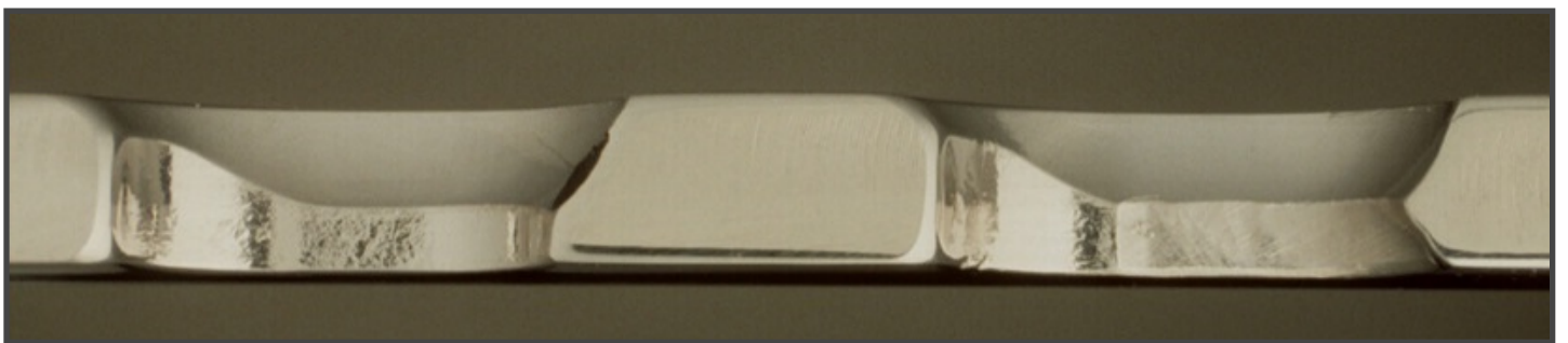
Fig. 13: DCP cut open, at the left the inclined slope allowing compression, the horizontal part allows gliding when a subsequent screw compresses.
