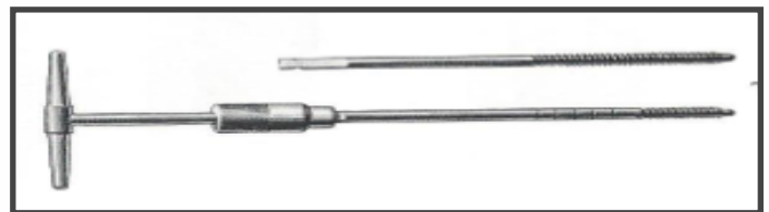
Fig. 6: Tap for precutting the thread which was identical to the one of the screw.
