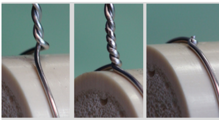
Fig. 9 Elastic and plastic deformation of the wire and breakage: increasing amounts of twisting torque applied result in the pictures from left to right. LEFT: too early release results in spring back. MIDDLE: proper plastic deformation. RIGHT: after breakage the traction in the wire may be maintained (Perren et al. 2011).
