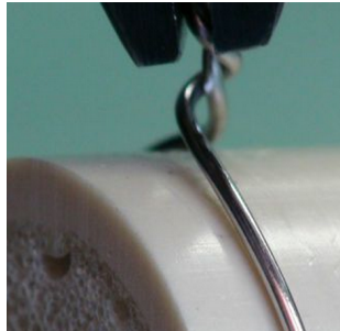
Fig. 21 Spring back situation when the wire is deformed only elastically and not plastically. The glossy appearance of the wire indicates absence of plastic deformation.
